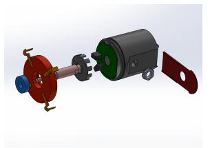
Image: An exploded view of the developed encoder.
